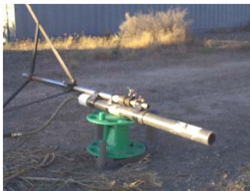
Figure 3. The propylene dissemination pipe (Photo by Chris Biltoft, WDTC).
