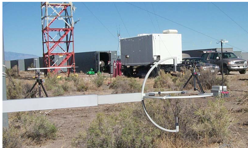
Figure 8. ATI Turbulence (Vx) array sonic with the VIP Van and 32-m tower in background. (Photo by Sam Chang, ARL).
