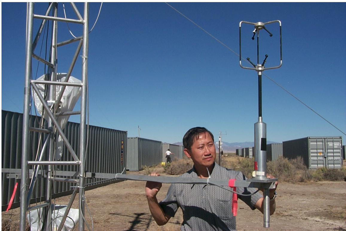
Figure 7. Young Yee with DSTL Gill Windmaster Sonic on 6-m tower (Photo by Sam Chang, ARL).
