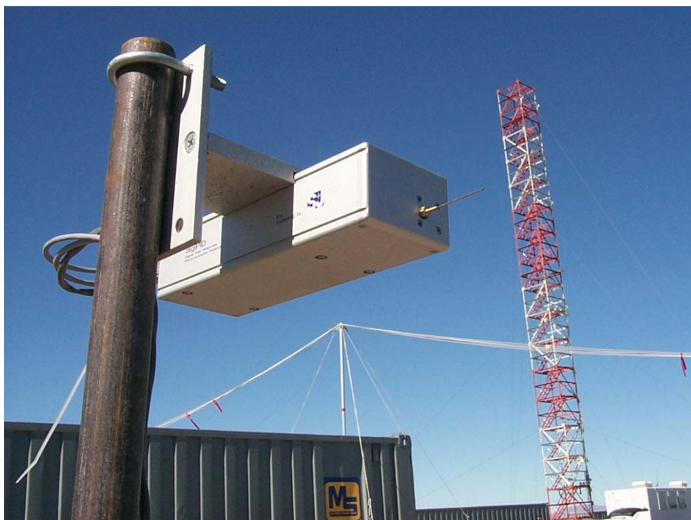
Figure 4. Digital photoionization detector (digiPID) mounted on stand with the 32-m tower in the background (Photo by Sam Chang, ARL).
