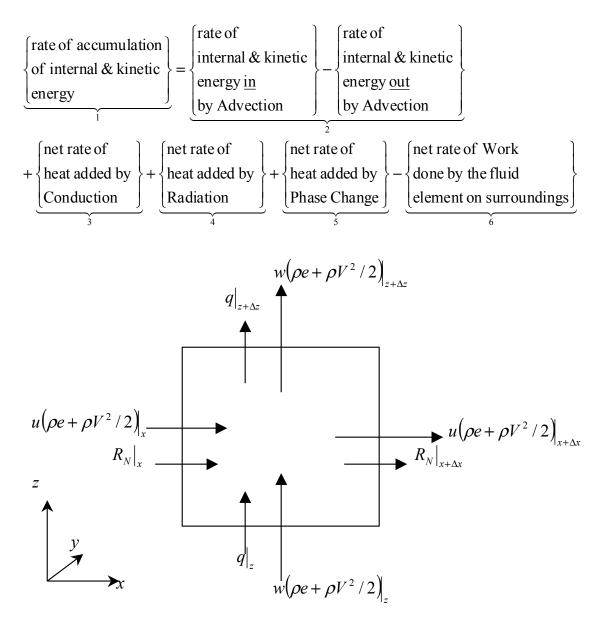
Figure 1: Schematic of a fluid element used for deriving the energy equation.
