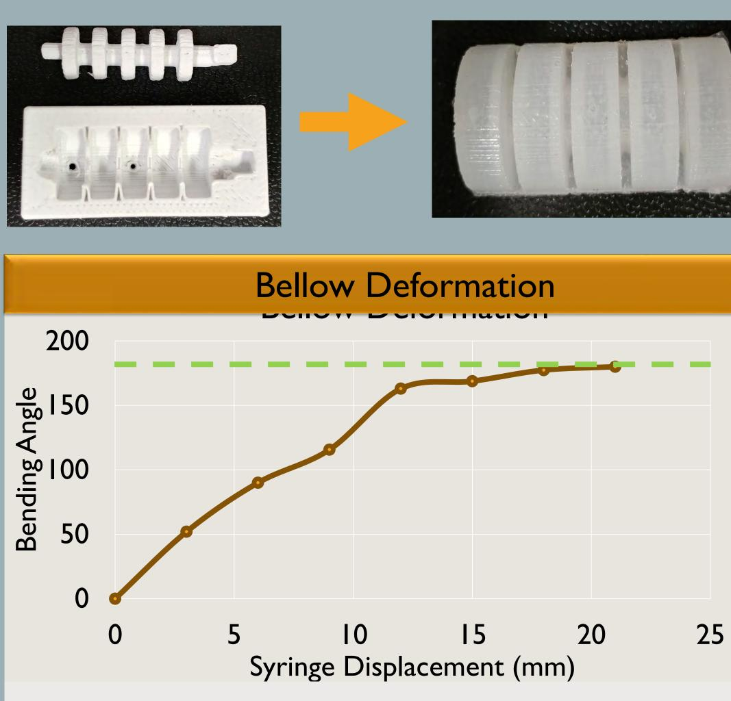
Specifications for the bellow design was to achieve an angle of up to 180° of deformation when attached to the syringe pump.
