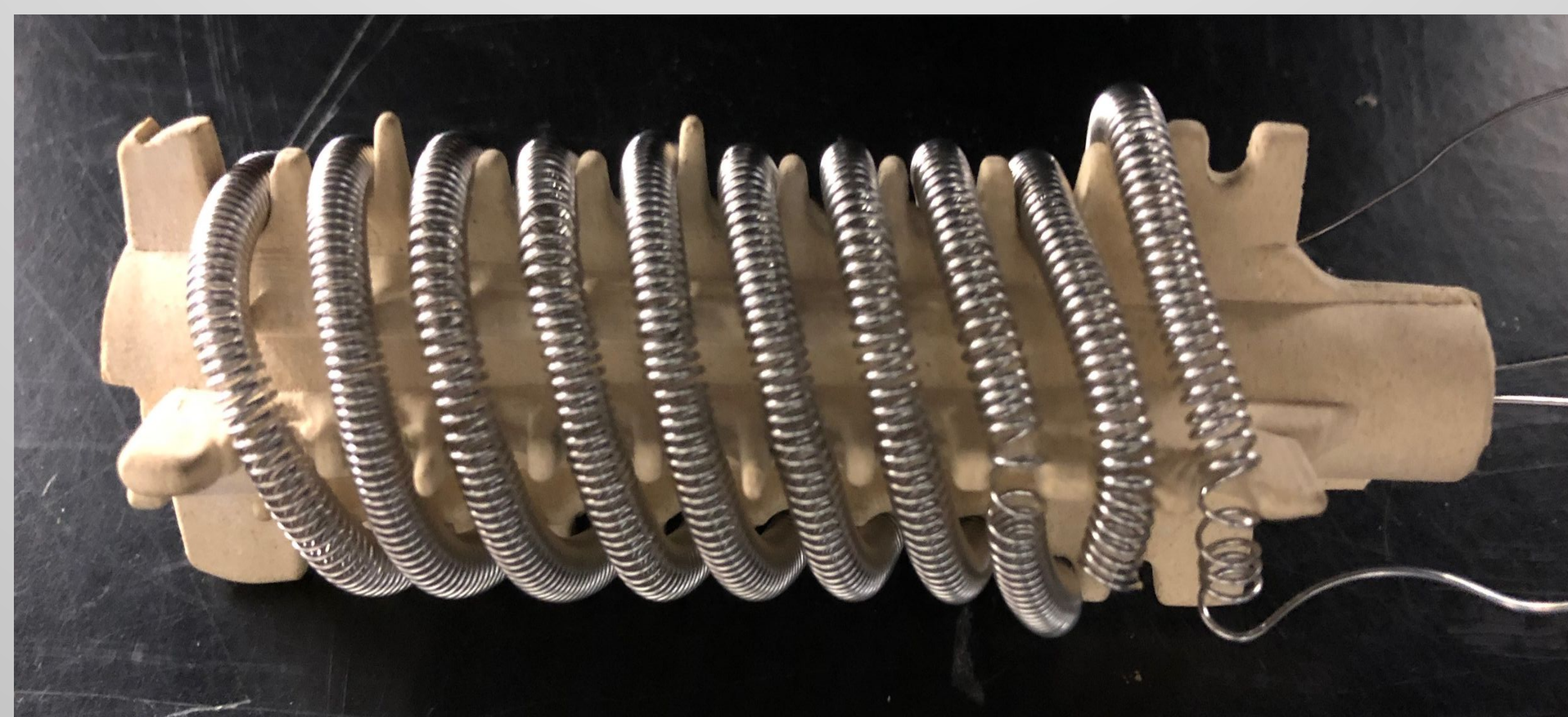
The heating element design which consists of two, 24-gauge nichrome wires coiled in a helical pattern around a ceramic core.
