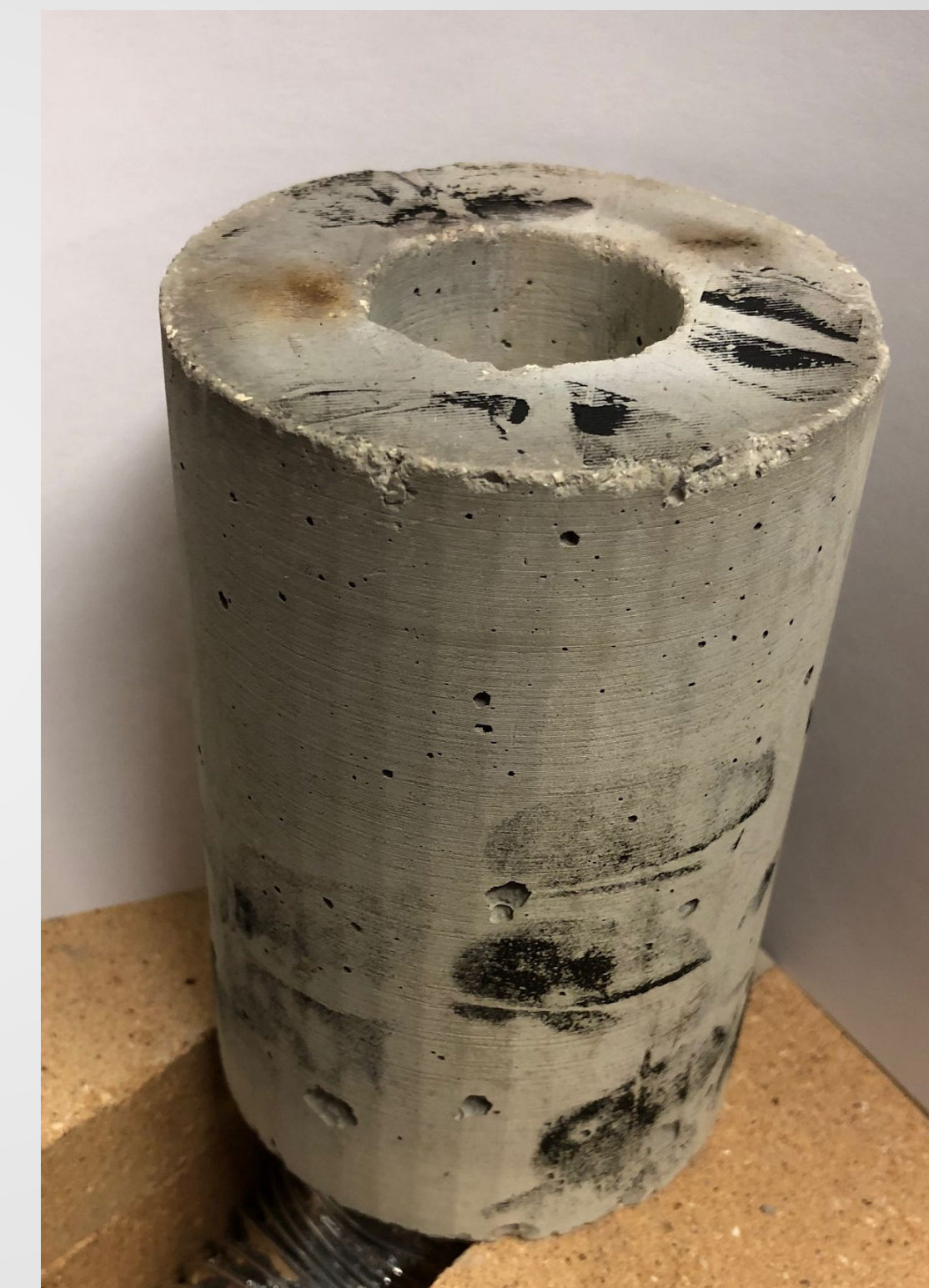
Firebrick chimney used to insulate the heating element.
