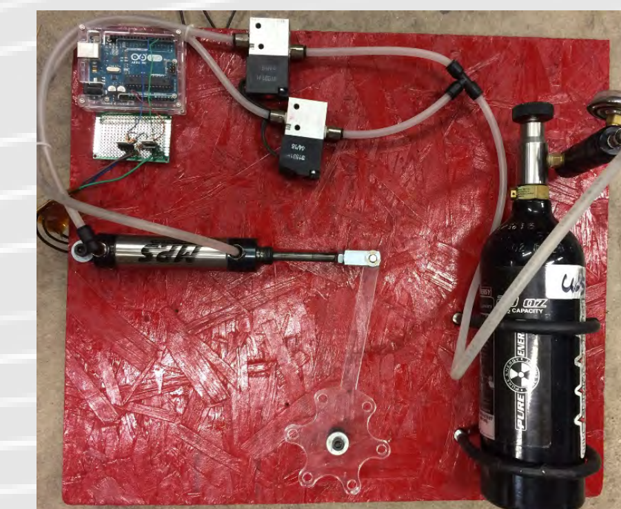
Actuator System mockup, showing all pneumatic components.
