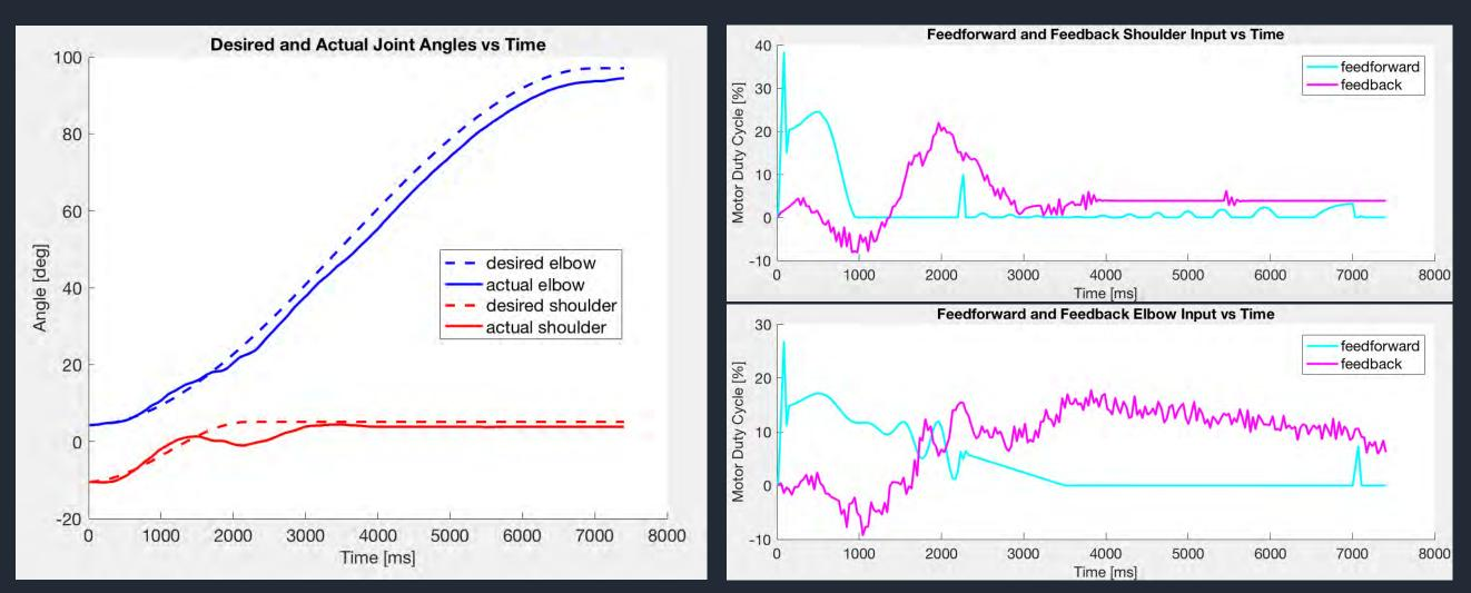
The left plot shows generated trajectories for the shoulder and elbow joints along with the actual trajectories that resulted from the RASM attempting to concurrently follow them. The two plots on the right show the feedforward and feedback control vs time for the shoulder and elbow joints that produced the actual trajectories in the left plot.
