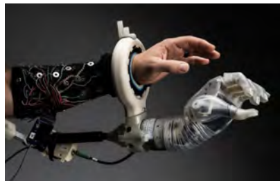
Assistant Professor Jacob A. George was named Innovator of the Year for his work with the “LUKE Arm”, a neuroprosthesis controlled by thought and endowed with a sense of touch.
