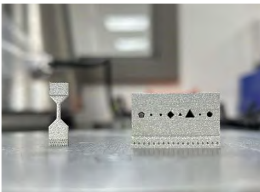
3D printed test coupon showing different channel geometries
