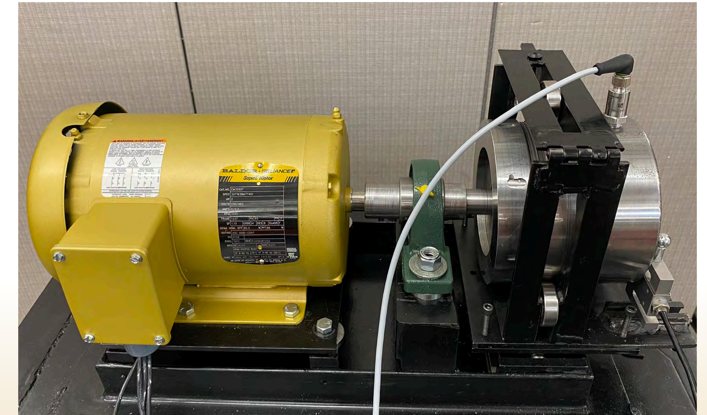
Figure 3: Manufactured test bench with tank, steady rest, shaft seal interface, purchased motor, and all sensors
