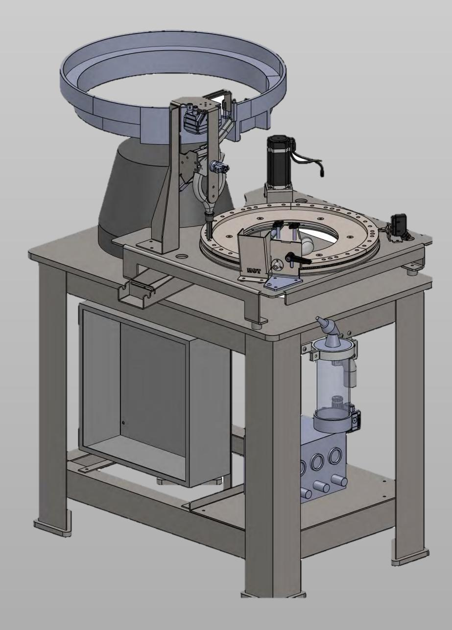
The assembly line consists of an alignment system with a vibratory bowl and a flipping mechanism. The broadheads then drop into a conveyor where they are transported to a heating chamber and a spraying chamber until they drop into a hole that sends them to a metal box and then into a bucket. The system is controlled by a programmable logical controller for autonomous movement. An example of the final product is shown below.
