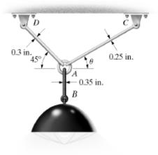
$$\stackrel{*}{\rightarrow} \Sigma F_x = 0; \qquad -T_{AD} \cos 45^\circ + T_{AC} \cos \theta = 0 \qquad (1)$$
