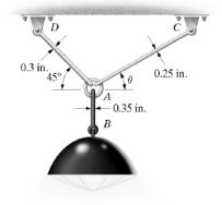
$$\begin{array}{l} \stackrel{+}{\to} \; \Sigma \; F_x = 0; \qquad F_{AC} \cos 30^{\circ} - F_{AD} \cos 45^{\circ} = 0 \\ + \uparrow \; \Sigma \; F_y = 0; \qquad F_{AC} \sin 30^{\circ} + F_{AD} \sin 45^{\circ} - 50 = 0 \end{array}$$
